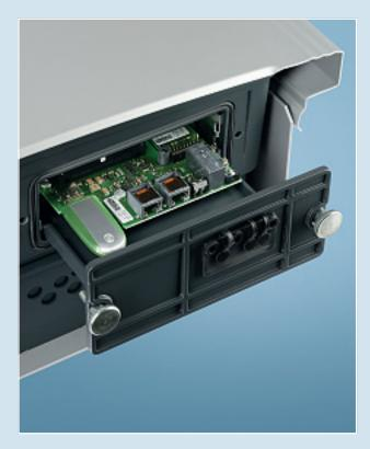
**DATCOM slot.** The DATCOM slot can be used for connecting the USB stick, optional DATCOM components as well as the direct signaling contact. It opens like a drawer providing easy access. Additional components can be connected later on as required.
